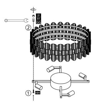
4. Remove the set screws on the fixture body
