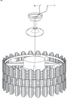
6 Install the screws into the motor cap
