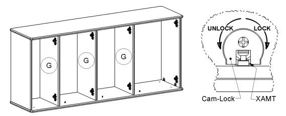
8. Evenly gap hardboard backs with each other and locate pre-drilled holes in the back edge of each Divider. Secure by installing 3-**XAED** 1-5/8" Drywall Screw through Hanging Brace and 3-**XCPT** Washer head Screws between Backs with a Phillips Screwdriver.
