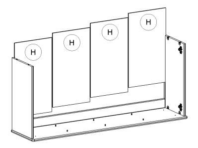
6. Install <u>Top</u>-**B** by aligning cam-locks with cam-lock bolts previously installed in Top and Backs resting in Top groove. Secure by turning cam-lock's metal center with a Phillips Screwdriver ¼ turn clockwise.
