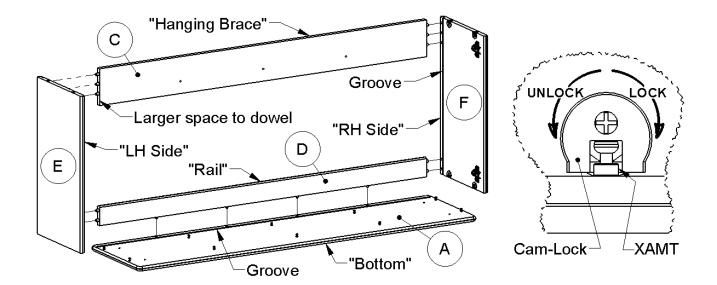
5. Drop in Backs-H into grooves on the Sides and Bottom.
