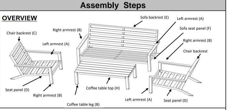
This product has multiple parts and may require up to 30 minutes to assemble. To give you an overview of the parts, the above picture is to help you put the various parts into perspective. Please read through the instructions below to familiarize yourself with the parts and steps before assembly.
