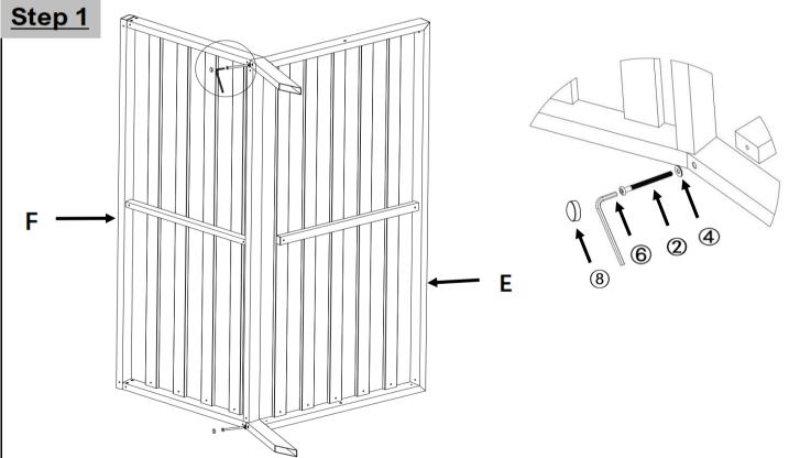
Place the Sofa seat panel (F) onto a clean, non-marring surface. Attach the Sofa Seat panel (F) with the Sofa backrest (E) as pictured, using Screws (②), Washer (④) and Spanner (⑥) and Screw Cover Cap (⑧).
