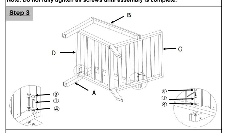
Attach the Armrest (A) with the Seat Panel and the backrest, using Screws (1), Washer (4) and Spanner (6) and screw nut (8) and Screw Cover Cap (8).
