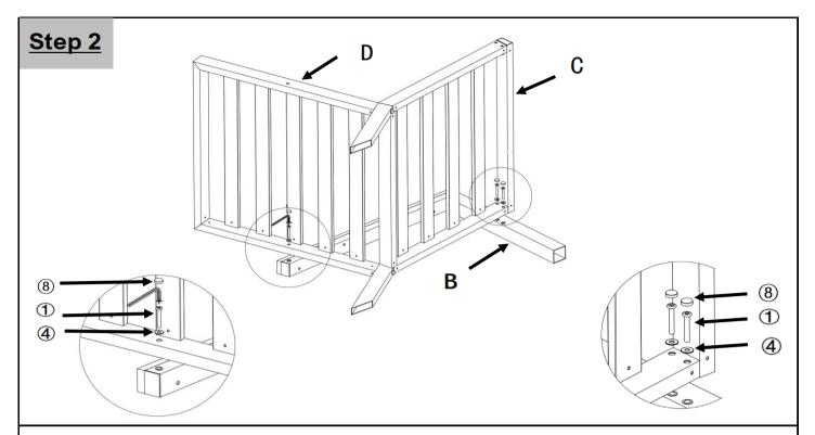
Attach the Armrest (B) with the Seat panel (D) and the backrest(C), using Screws (1), Washer (4) and Spanner (6) and Screw Cover Cap (8).
