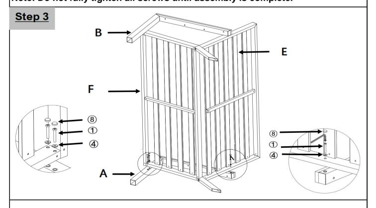
Attach the Armrest (A) with the Sofa seat panel (F)and the Sofa backrest(E), using Screws (1), Washer (4) and Spanner (6)and Screw Cover Cap (8).
