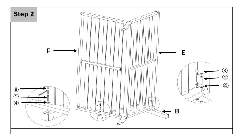
Attach the Armrest (B) with the Sofa seat panel (F) and the Sofa backrest (E), using Screws (1), Washer (4) and Spanner (6) and Screw Cover Cap (8).
