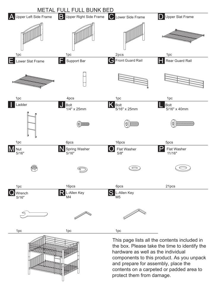
Attach Upper Left & Right Side Frame (A & B) to Upper Slat Frame (D) using Bolt (K), Spring Washer (N) and Flat Washer (P) with L-Allen Key (S). Attach Lower Side Frame (C) to Lower Slat Frame (E) using Bolt (K), Spring Washer (N) and Flat Washer (P) with L-Allen Key (S).
