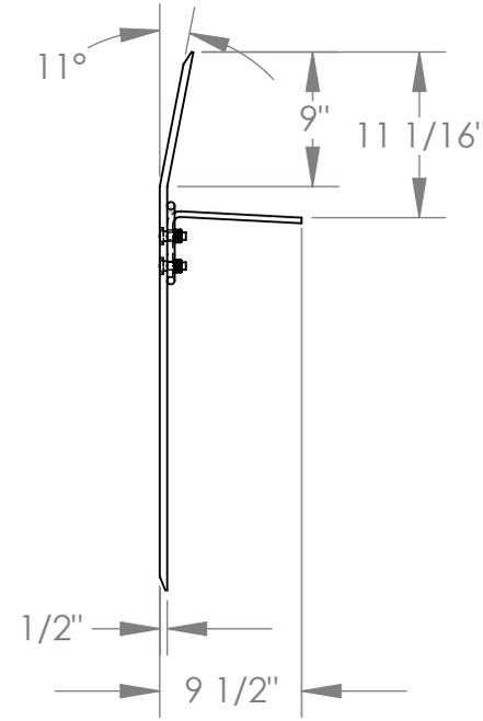
NOTE: BEND OR CROWN IS 11° AND LOCATED 9" FROM EDGE OF DOCKPLATE
