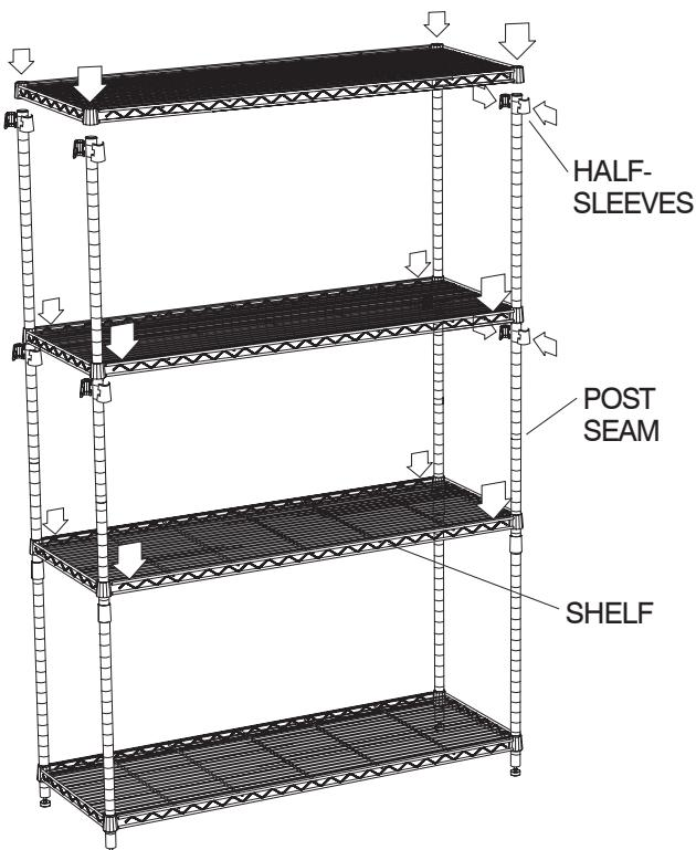
**6** Connect optional add-on upper posts to lower posts using step 1. Install half-sleeves for bottom add-on shelf, refer to step 2. Insert posts into short side of add-on shelf referring to steps 3 and 4. Slide two E-S-Connecting Hooks onto each front frame of starter unit shelves. Position hooks at least 12 inches apart.
