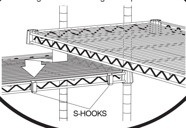
**7** Snap half-sleeve sets onto add-on posts at same height as next shelf on starter unit. Lower the next shelf into position with the shelf frame of the non-post side on the S-hooks. Press corners near half-sleeves until fully seated. Install the third and fourth shelves in the same manner.
