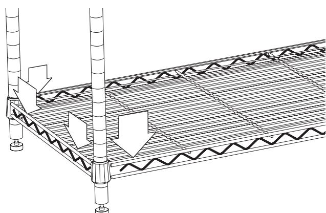
**5** Snap half-sleeve sets onto all four posts at desired height for next shelf. Lower next shelf into position and press until fully seated. Install third and fourth shelves in the same manner, with both shelves mounted ABOVE the post seams.
