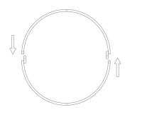
6.Put the iron ring into the lamp body and lock them with screws.
