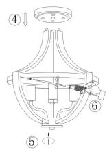
4.Align the hole on the disc with the flat bar, then clip it in and lock it with a nut.
