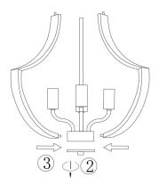
2.Loosen the ball nut under the lamp body.
