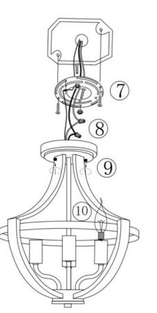
7.Attach the cross bar to the outlet box by using two mounting Screw.
