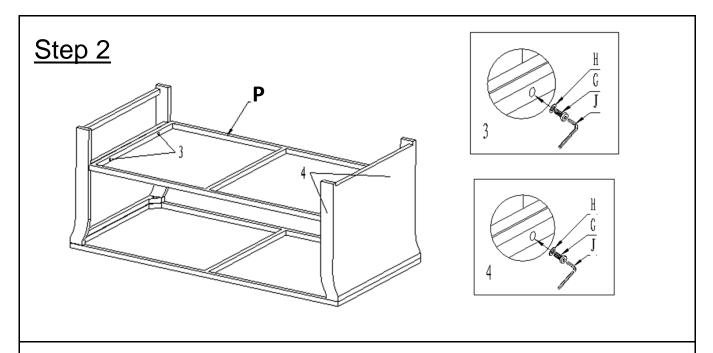
Attach the Table Shelf(P) between the two Table Legs(R) using Hardware(H, G) with Allen Key(J) as shown in Picture 3 and Picture 4.
