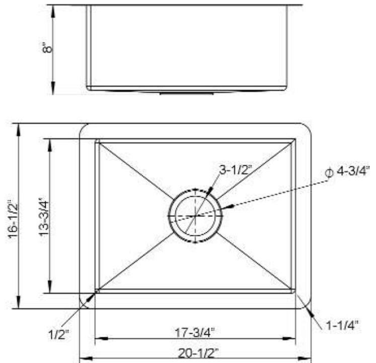
Dimensions of fixture are nominal and may vary within the range of tolerances established by ANSI Standard A112.19.2. Dimensions and specifications subject to change without notice.
