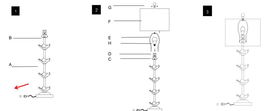
Step 1 Be careful not to twist the power cord and tighten securely
