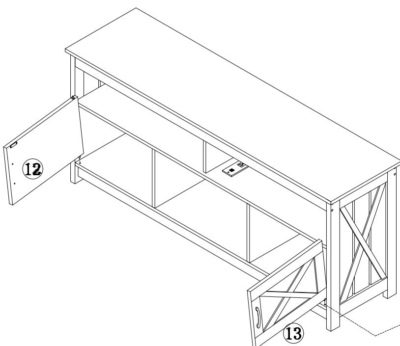
Note: As shown in the picture below, please press down the shrapnel shaft by hand, align the shrapnel shaft with the pre-drilled hole and release it.
