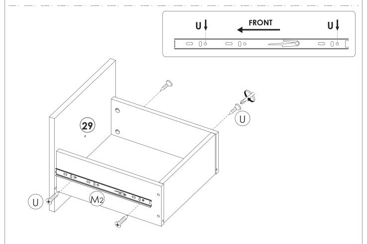
**REMARK:** Align the slides and push the drawer carefully inside until it stops.
