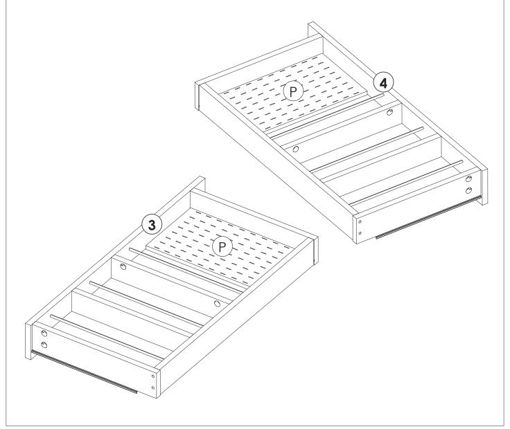
**REMARK:** Align the slides and push the drawer carefully inside until it stops.
