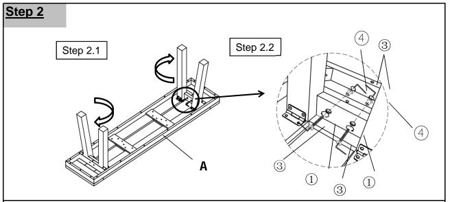
Place the Bench (A) facedown, onto a clean, soft surface to avoid any scratches or damage to the product.
