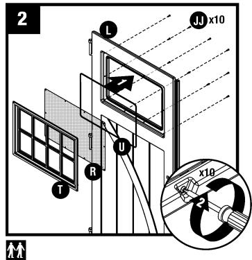
Place gasket (U), window (R), and frame (T) into door channel. Secure with ten screws (JJ), starting at corners. **DO NOT** over tighten screws. Repeat for right door (M).
