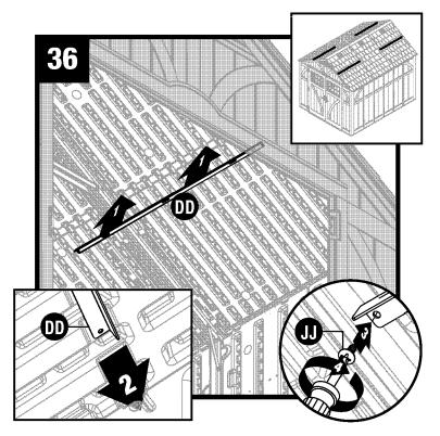
Raise roof support bracket (DD) into position against roof. Slide roof support bracket (DD) into front header. Secure roof support bracket (DD) to underside of truss leg with one screw (JJ).
