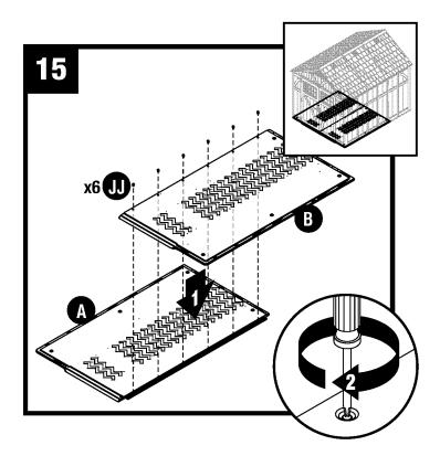
Push left floor (A) and right floor (B) panels together and secure with six screws (JJ).
