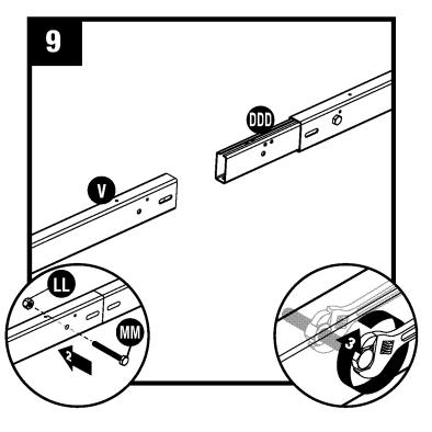
Place 7' ridge beam (V) onto the ridge beam joiner (DDD). Secure with hex bolt (MM) and nut (LL).
