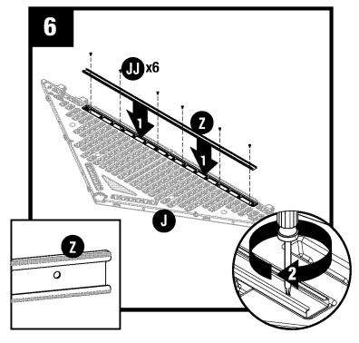
Place header beam (Z) into pocket of front header (J). Secure with six screws (JJ). **DO NOT** over tighten screws.
