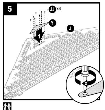
Lay front header (J) on ground with lettering side facing up. Place fiberglass vent screen (Y) into rear opening in front header (J). Secure with eight screws (JJ). **DO NOT** over tighten screws.
