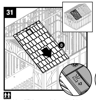
Slide right roof (O) down towards the outside of shed.
