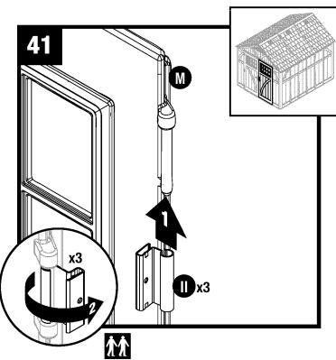
Stand right door (M) upright with three hinge mounts facing right. Slide one metal door hinge (II) up onto each hinge mount. Rotate door hinges to outside of door.
