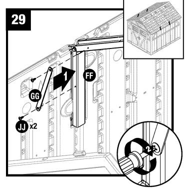
Attach truss strap (GG) to side adaptor bracket (FF) with two screws (JJ).
