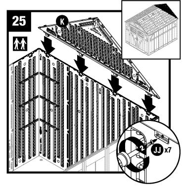
Place rear header (K) over back walls and fit four protruding support legs into pockets molded in back walls. Secure rear header using seven screws (JJ).
