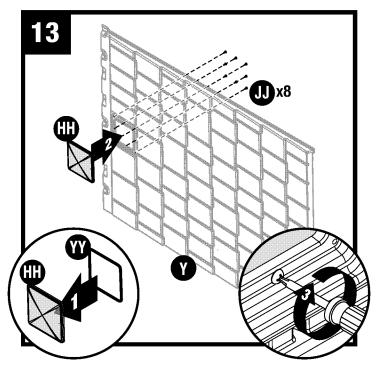
Place skylight gasket (YY) into skylight (HH). Place skylight (HH) onto right roof panel (O). Secure from underside with eight screws (JJ). Make sure rib on plastic parts is seated fully against gasket on skylight.
