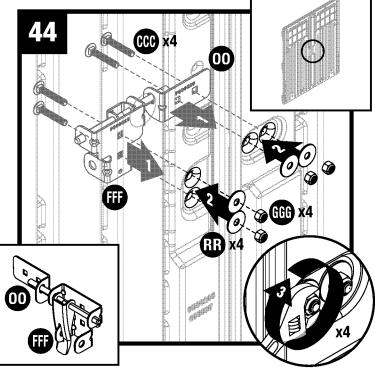
Insert two screws (CCC), into left latch plate (OO), and through pre-drilled holes in doors. While holding plate in place on exterior door, secure with two washers (RR) and two locking nuts (GGG). Repeat for right latch plate (FFF).
