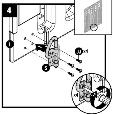
At bottom interior side of left door (L), attach D-ring slide bolt (S) with four screws (JJ).
