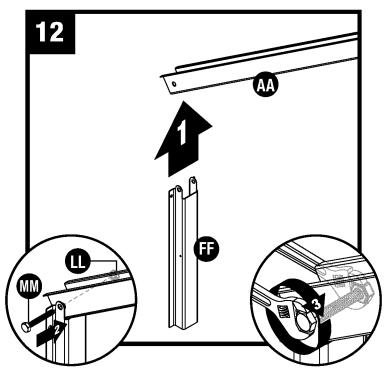
Attach side adaptor bracket (FF) at end of left truss leg (AA) with one cap screw (MM) and one nut (LL).
