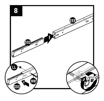
Place ridge beam joiner (DDD) into the 3' ridge beam (EEE). Secure with hex bolt (MM) and nut (LL).
