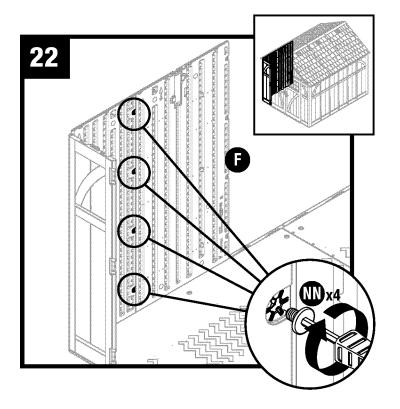
Secure side panel (F) with four easy bolts (NN), working from floor to roof. **DO NOT** use torque wrench. Use easy bolt easy driver (OO) and hand tighten. Easy bolt head will be flush when fully seated. **DO NOT** over tighten easy bolts.
