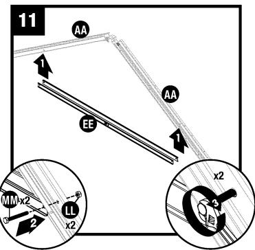
Attach two truss cross beams (EE) to two truss legs (AA) with two cap screws (MM) and two nuts (LL). Stand truss and check cross beam is level.
