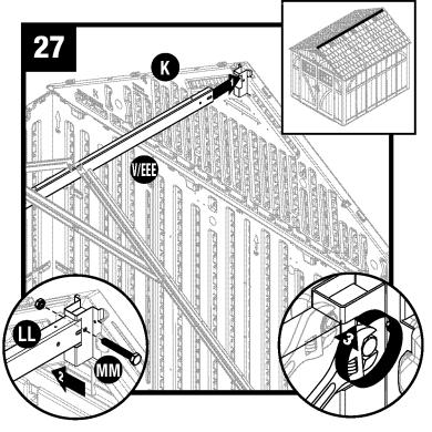
Raise ridge beam (V/EEE) up and into rear header (K). Secure with one bolt (MM) and one nut (LL). DO NOT tighten. Repeat for front header (J).
