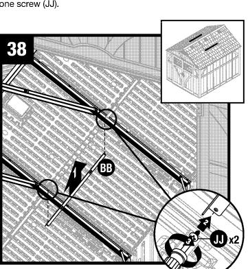
Attach roof support extension (BB) to truss legs with one screw (JJ), each side.
