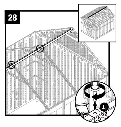
Attach the roof truss assembly to the ridge beam with two screws (JJ).
