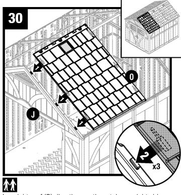
Lay right roof (O) directly over three tabs on right side of front header (J). With right roof slots seated over/on header tabs, check alignment in all three spots.
