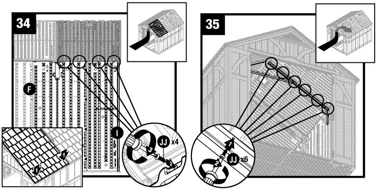
Pull down each lower corner of roof from outside. From inside shed, attach tabs on right front corner (I) and side panel (F) to roof panel with four screws (JJ).
