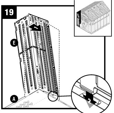
Tip left front corner (E) back to vertical position and align lower tabs on right side with slots in floor.
