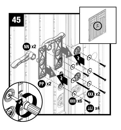
From the outside of doors, insert door handles (NN) onto the handle plates (PP). On inside of the doors, place washers (HHH) on center door handle locations, and secure each handle (NN) with one long screw (KKK).
