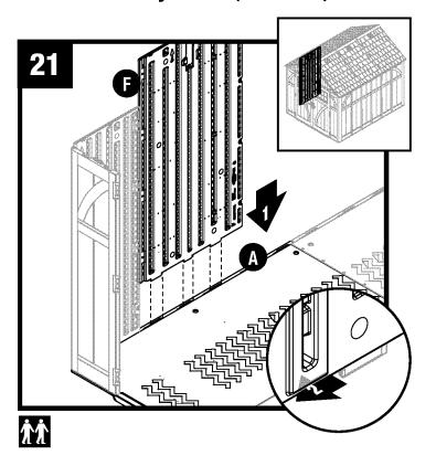
Align tabs on bottom of side panel (F) with slots along floor (A). Lower panel into slots and lock in place by sliding panel toward front corner.
