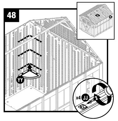
Attach shelf (YY) in desired location with four screws (JJ) Repeat for remaining shelf (YY).
