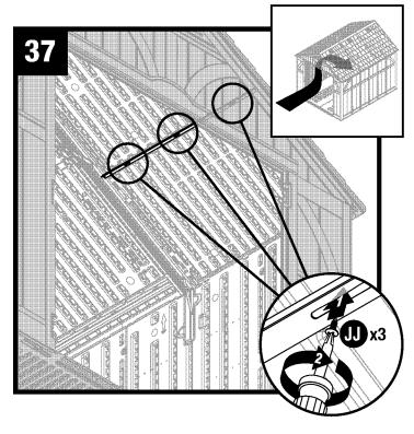
Secure roof support to roof using three screws (JJ).
