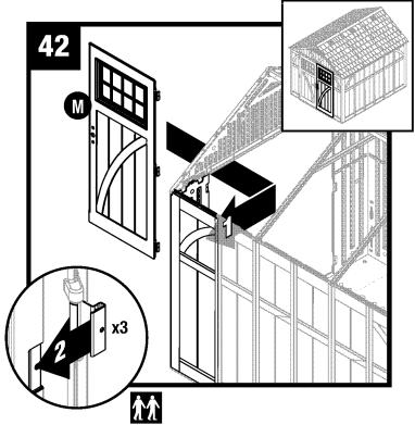
With door hinge in open position, slide one door hinge over each hinge receptacle on inside of right front panel.
