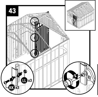
Secure each metal hinge plate with one screw (KK) and one nut (LL).
