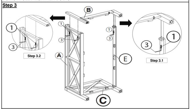
Place Left Arm Panel (B) onto the assembled frame from Step 2
