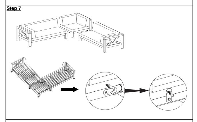
Note: This is optional step in case we want to connect all chairs in a set together and should be done before placing cushion
