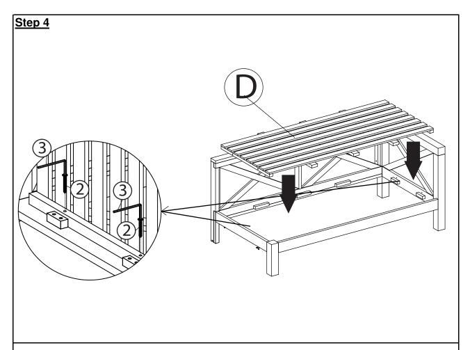
Attach the Seat Panel (D) into the Right Chair as shown in picture above.
