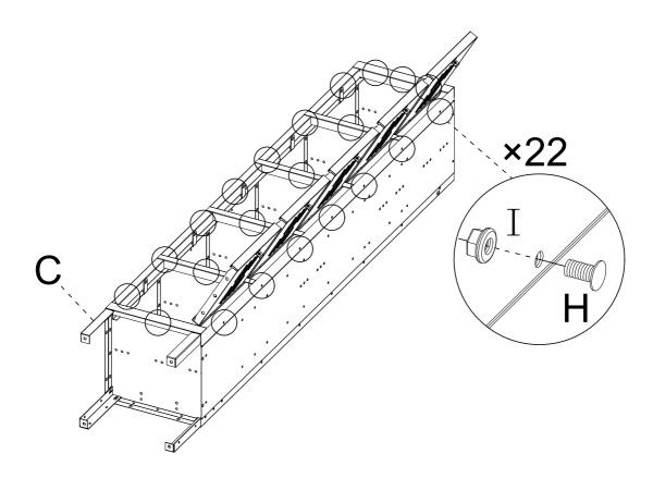
Snap on the door panel and install the nuts from the inside.
