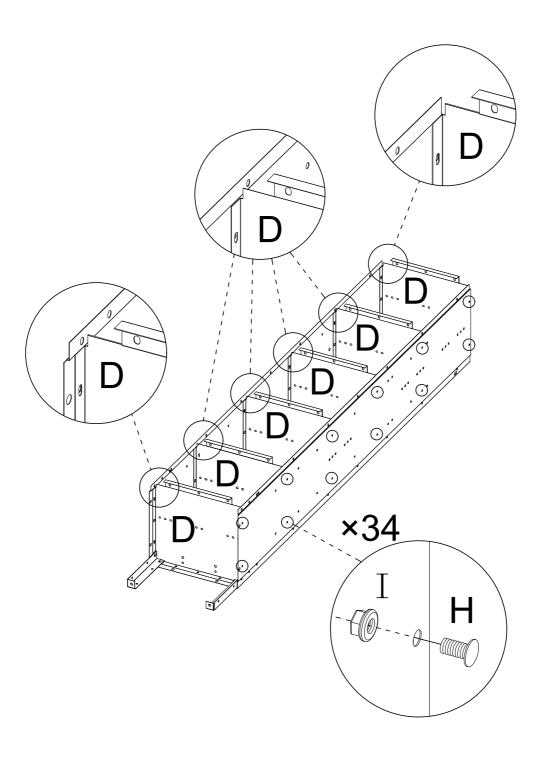
Assemble 6 Parts D, back plate B and side plate A with H\*34 bolts and I\*34 nuts
