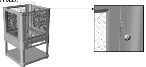
STEP 6: Connect the Hood (B) to all screen by using M6 \* 10 Bolt (AA).
