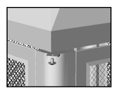
STEP 7: Insert the Handle (H) into the hole in the Door screen (F) using M6 Nut (BB).
