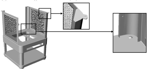
STEP 5: Connect Back screen (C) to the Left screen (E) and Right screen (D) with M6 \* 10 Bolt (AA), connect Door screen (F) to Left screen (E) and Bracket (I) with M6 \* 10 Bolt (AA). **TIGHTEN ALL BOLTS FULLY.**
