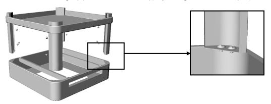
STEP 4: Turn the Base (M) with Bracket (I) in the upright position, connect Left screen (E) and Right screen (D) to the Bracket (I) with M6 \* 10 Bolt (AA). **DO NOT TIGHTEN THE BOLTS FULLY.**
