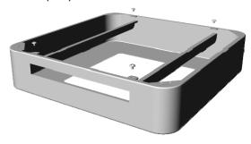
STEP 3: Connect 4 Legs (L) with the Bracket (I) by using M6 \* 10 Bolt (AA).
