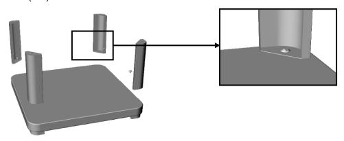
STEP 2: Reverse the Bracket (I) and then connect the Ash pan orbit (K) to the Bracket (I) by using M6 \* 10 Bolt (AA).
