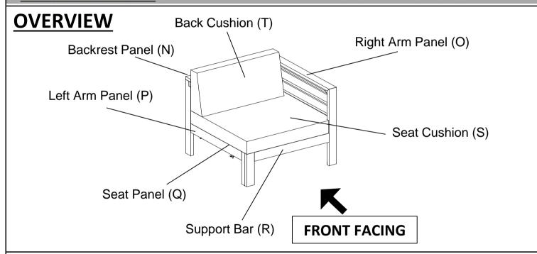
This Right Chair has multiple parts and may require up to 30 minutes to assemble. To give you an overview of the Right Chair parts, the above picture is to help you put the various parts into perspective. Please read through the instructions below to familiarise yourself with the parts and steps before assembly.
