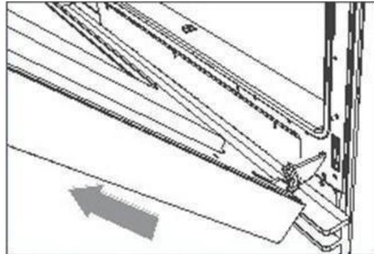
4. Disengage the hinges and remove the gently close it about halfway. door, place on a protected surface.
