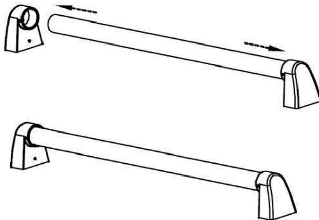
3.3 Secure the oven handle with two screws on each door handle holder (if not, handle might be loose)
