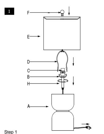
Pull power cord to connect the Neck (H) to the Base (A) Insert the Harp (D) into the Saddle (B).
