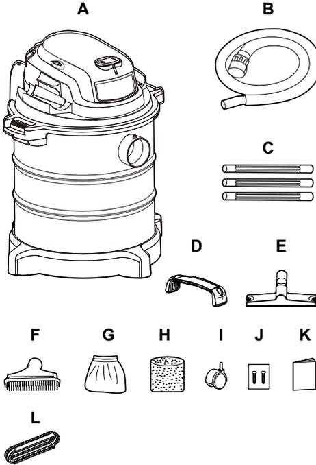
Remove all contents from the box. Remove the power head and take out any contents inside the collection tank. Check each item against the carton contents list.
