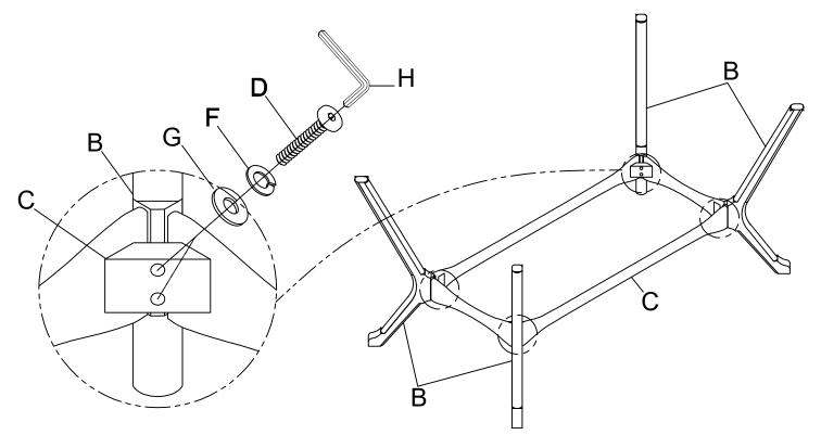
Attached Leg Frame(C) to the Table Top(A). Use Allen Bolt(E) Lock Washer(F) and Flat 2 Washer(G) on holes of Table Top(A). Turn the Allen Key(H) in Allen Bolt(E).
