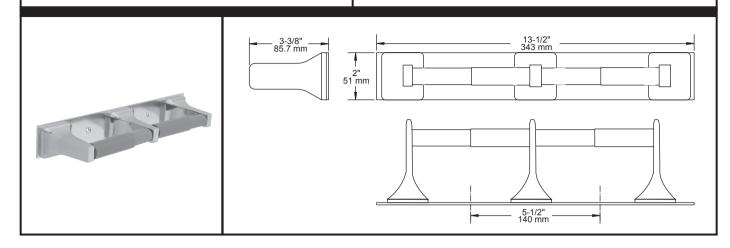
MATERIALS: Paper holder posts are die cast from highest quality virgin zinc alloy (Zamak) to meet ASTM standard B-86.
