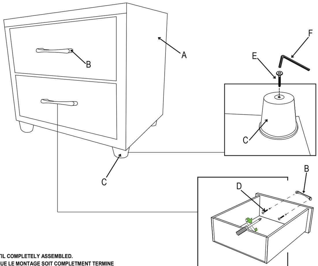
DO NOT TIGHTEN BOLTS UNTIL COMPLETELY ASSEMBLED.
