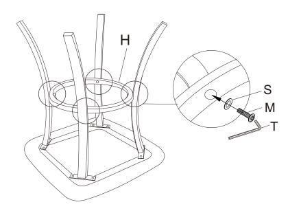
Place part H upside down, align with the reserved hole of part P, put the screw M over the gasket S, and lock it with the hex tool T.
