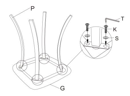
Place table G upside down, and flat, align table foot P with the reserved hole on table G, insert gasket S with screw K, and lock it with hex socket tool T.
