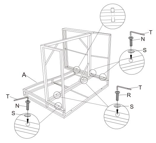
Lay the right armrest A flat and align it with the reserved holes in accessories D and C,Use the corresponding screws N and R to cover the gasket S and lock it tightly with the hex tool T.
