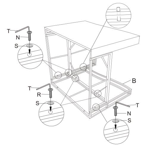
Lay the left armrest B flat, align it with the reserved holes in accessories D and C, cover the gasket S with the corresponding screws N and R, and lock it with the hex socket tool T.
