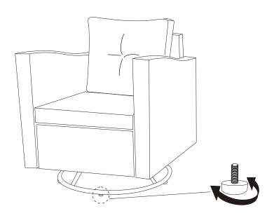
If the turntable is not level after the assembly of the turntable, there is a shaking phenomenon you can adjust by rotating the plastic nail at the bottom of the turntable to make the chair stable.
