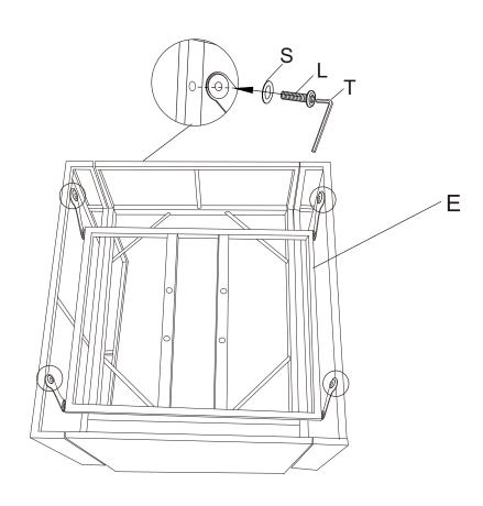
Place the upper seat assembled in step 3 upside down, place part E in the bottom, align the holes reserved for parts A and B, cover the gasket S with screw L, and lock it with the hex socket tool T.
