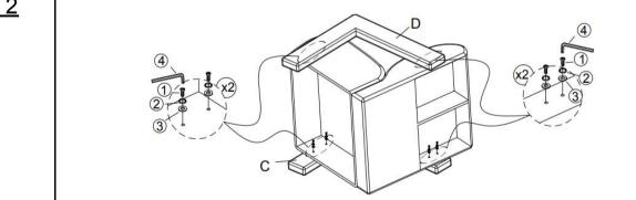
Attach Left Arm(C) and Right Arm(D) to Seat Frame(A) and Backrest Frame(B) by using Bolt (1), Spring Washer (2), Flat Washer (3) and Allen Wrench (4), as pictured above.
