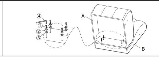
Attached Seat Frame (A) to Backrest Frame (B) by using Bolt (1), Spring Washer (2), Flat Washer (3) and Allen Wrench (4), as pictured above.
