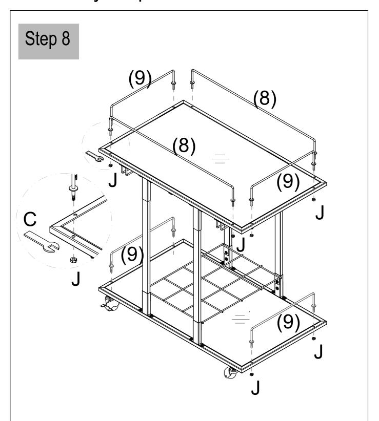
Attached Long Rail Bar (8) and Short Rail Bar (9) to the Top Frame (1) and Bottom Shelf Frame (2), Secure with Nut J by using a Small Wrench C.
