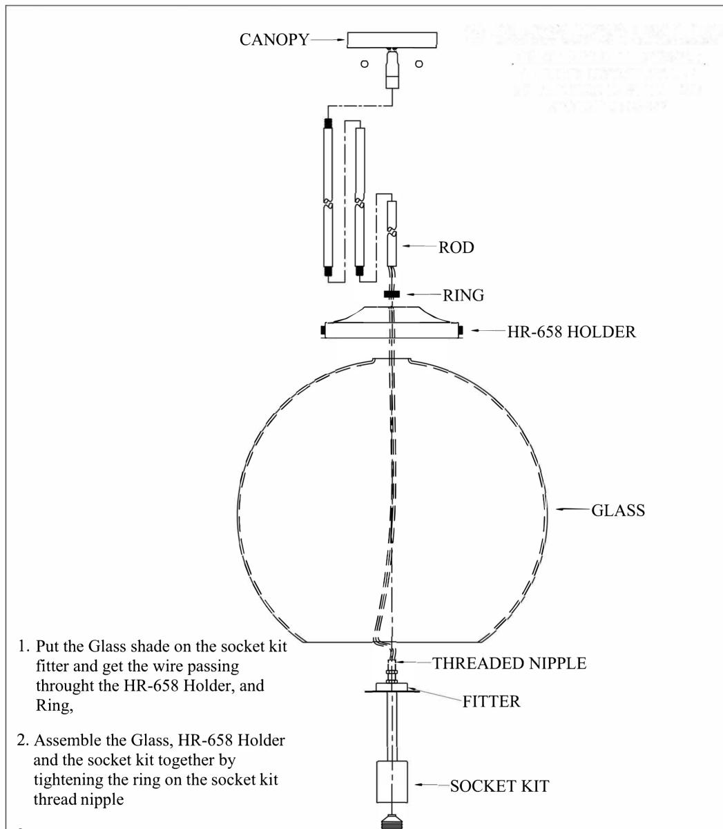
3. Passing the wires through the rods and get rods assembled onto the top threaded nipple in getting your desired height, then, assemble the canopy.
