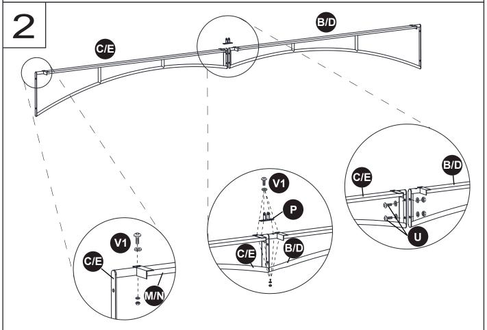
Fix Left Lintels (B/D) with Right Lintels (C/E) with Screw (U) , Fix U-Shaped Connector (P) and Screen Rod (M/N) on lintels with Screw (V1) ;
