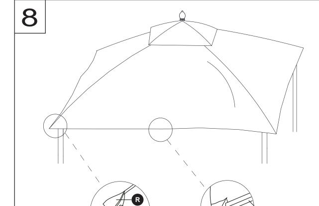
Tighten the fabric cover (R) by pulling over the four small connector poles as shown.
