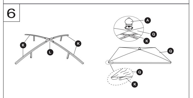
Insert each small top bar (K) into the small center connector (L). Attach the small roof (Q) on the small top bar (K), then secure with the decoration ball (A);
