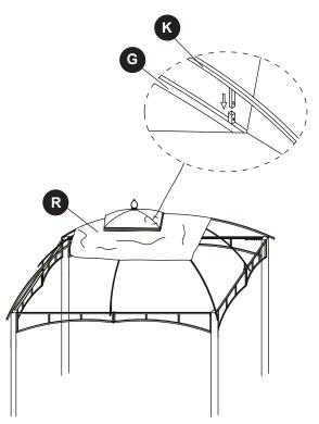
Place the fabric cover (R) loosely on top of the assembly. Insert each small top beam (K) into the long top connector pole (G).
