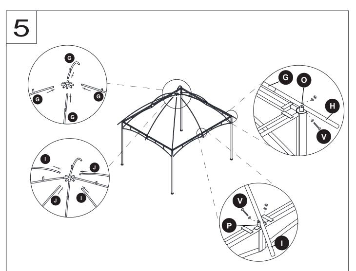
Insert Long Top Bar Tube (G) and Short Top Bar Tube (I/J) into Center Connector (A) ,Fix Short Bart Tube (I) on Middle Beam Down Connector (P) with screw (V) , Fix Long Support Connecting Tube (H) with U-Shaped Connector (O) with Screw (V) ;
