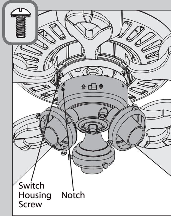
Partially install two of the switch housing screws found in the ≡ bag. Align the notches in the sides of the lower switch housing with the upper switch housing screws. Twist the lower switch housing clockwise to lock into place.
