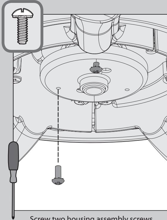
⊗ Screw two housing assembly screws from the
