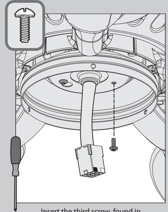
⊗ Insert the third screw, found in the
