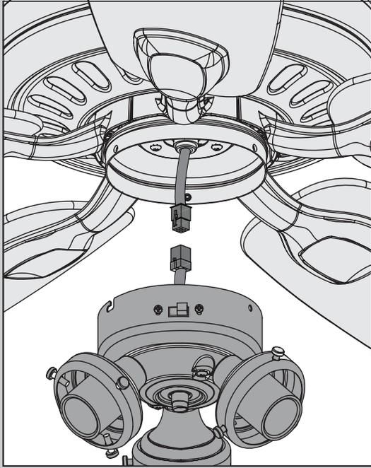
Connect the plugs from the upper and lower switch housings. Make sure to line up the colored markings on the connectors.
