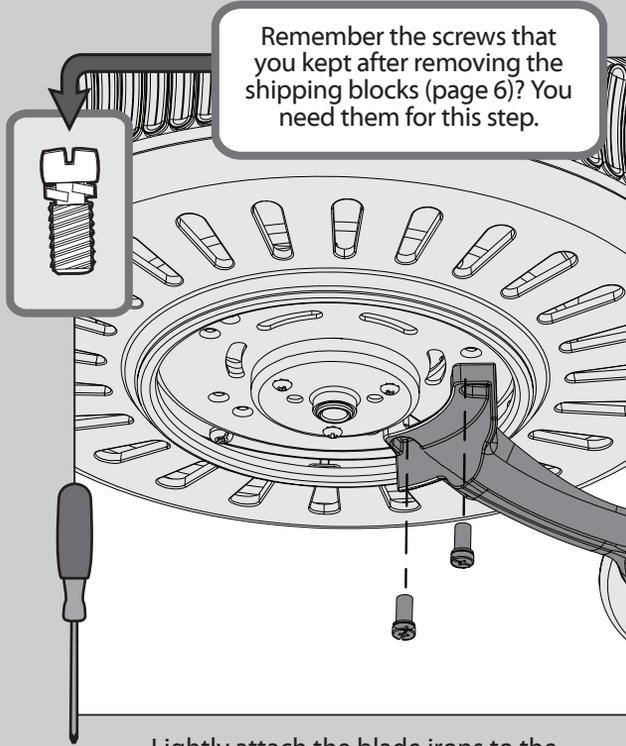
⊗ Lightly attach the blade irons to the motor with the blade iron armature screws, then securely tighten after both screws are attached.
