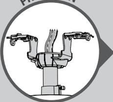
Using an orange wire connector from the ★ hardware bag, connect the 3 grounding wires (green, green/yellow stripe, or bare copper) coming from the ceiling, downrod, and hanging bracket.
