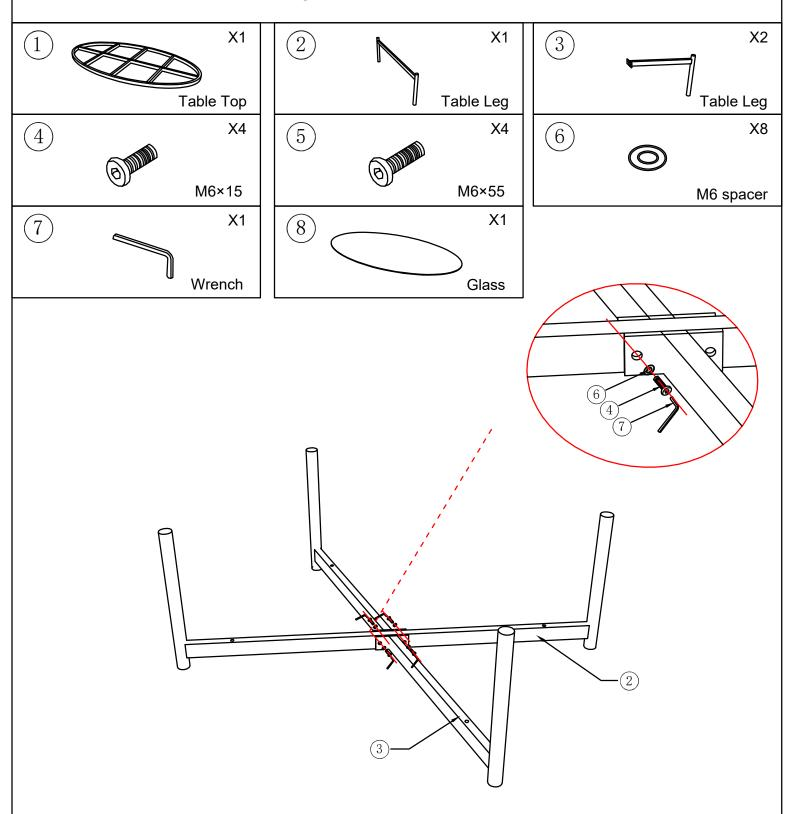
Step 1: Align the screw holes of the table leg(2) with the screw holes of the table leg(3), insert flat washers(6) and screws(4) into each hole, once the screws are in place, tighten the screw until firmly attached with the wrench provided.
