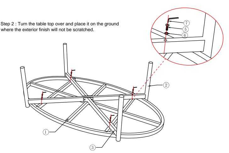
Step 3: Align the screw holes of the table legs with the screw holes of the table top, insert flat washers(6) and screws(5) into each hole, once the screws are in place, tighten the screw until firmly attached with the wrench provided.
