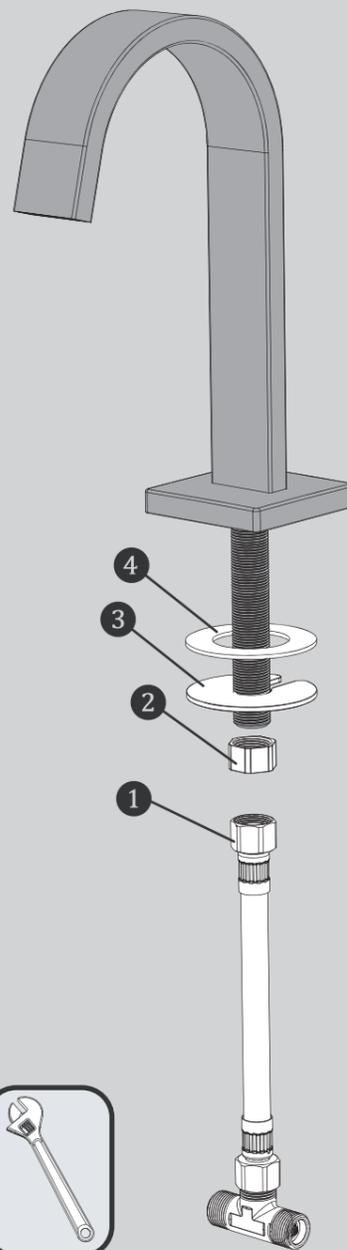
**2** Remove Mounting Nut (1), Metal Washer (2), and Rubber Washer (3) from Cold Endbody Assembly. Repeat process for Hot Endbody Assembly.
