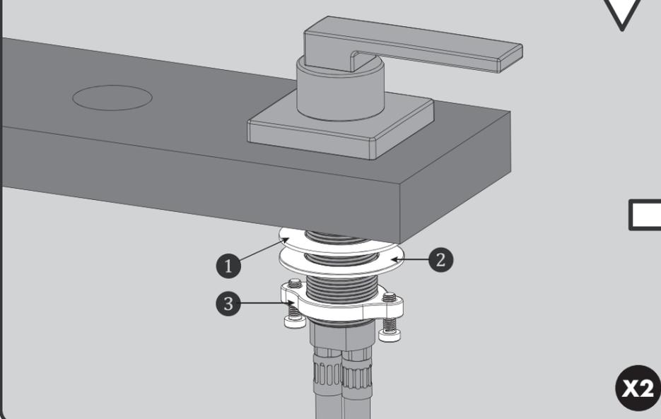
**5** Place Spout Assembly through the center hole of counter top. From below, reinstall the Spout Rubber Washer (1), Metal Washer (2), and Mounting Nut (3). Loosely assemble at this time. Reinstall Inlet Hose Assembly (4)
