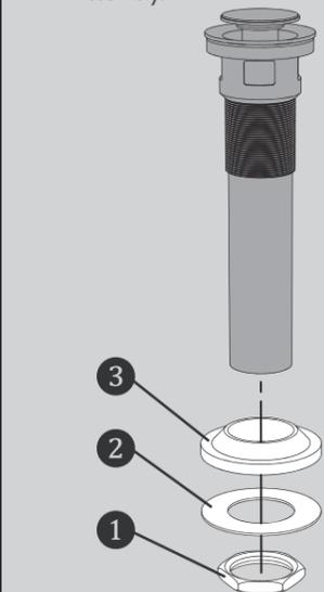
**11** Apply included Upper Drain Seal (1) or Plumber's Putty to the underside of the Upper Flange. Insert Drain Assembly into drain hole of sink from above.
