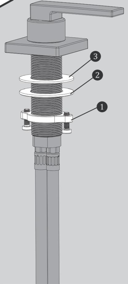
**3** The "COLD" and "HOT" Endbody Assemblies are clearly marked. Place COLD Endbody Assembly through the appropriate hole in the counter top. Align Endbody Assembly so the Rubber Access Plug (1) is facing the rear. Repeat process for the HOT Endbody Assembly.
