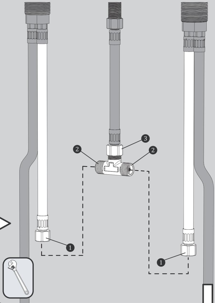
**9** Make connections to water supplies. The inlet threads of the faucet are 9/16"-24 UNEF and will accept a 3/8" Compression Fitting. Wrench Tighten.
