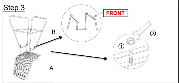
Align the mounting positions on Chair Leg(B) and Chair Seat(A), then attach using Nuts(①) with Spanner(②).
