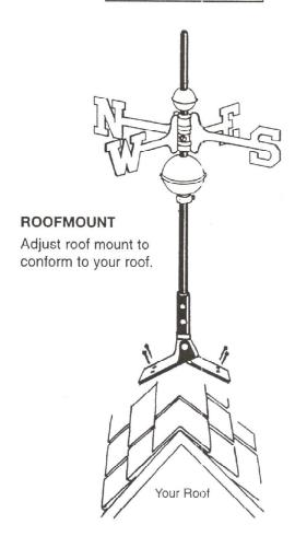
Drill 3/32" holes using roofmount as a template. Fill holes with silicone caulk and drive in 1 1/4" screws provided. Check
