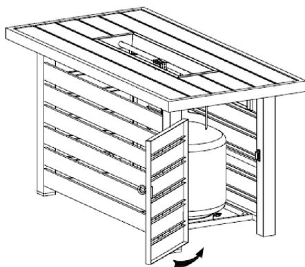
Load the Gas Tank / Gas Cylinder as indicated by the bold black arrow.
