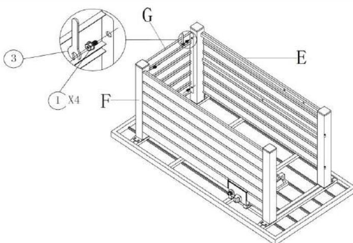
3. Attach panel (G) with panel (E) and panel with window (F) together using 4pcs of Bolts(①) with Allen Key(③). Pls do not fully tighten.
