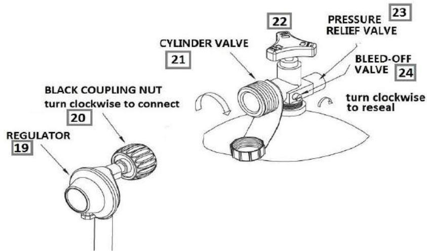
4. Turn the Cylinder Valve (21) on the tank in a clockwise direction to **TURN OFF SUPPLY** of the LP Gas supply . Attach the preassembled Regulator (12/19) from the Fire Table / Column to the Cylinder Valve (21) by turning the Black Regulator Coupling Nut (20) clockwise. Make sure it is fastened securely and tighten connections - by **HAND** only.
