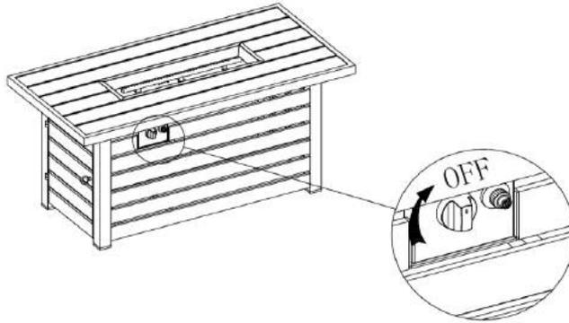
1. Check that the Control Knob (13) for the gas supply system is turned to the “OFF” position before starting any assembly.
