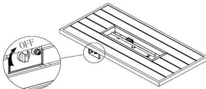
1. Check that the Control Knob (13) for the gas supply system is turned to the “OFF” position before starting any assembly.
