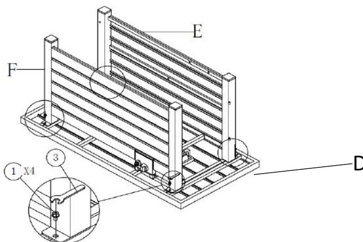
2. Attach panel (E) and panel with window (F) to the bottom of table top (D) using 4pcs of Bolts(①) with Allen Key(③). Pls do not fully tighten.
