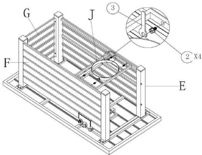
5. Attach metal stand (J) to metal base using 4 pcs of Bolts(②) with Allen Key(③). And tighten all Bolts.
