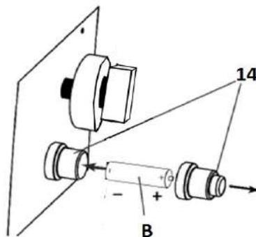
6. Remove the Electronic Ignitor Cap (14) on the electronic Ignitor (14) by unscrewing and slide the Battery (B) into the battery slot (14). Make sure the positive side of the Battery( B ) faces outwards. Screw the Electronic Ignitor Cap (14) over the battery, tightly.
