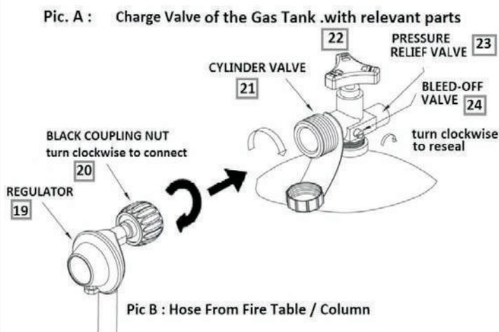
**Step 1 : Plug the Black Coupling Nut on the Regulator to the Cylinder Valve.**
