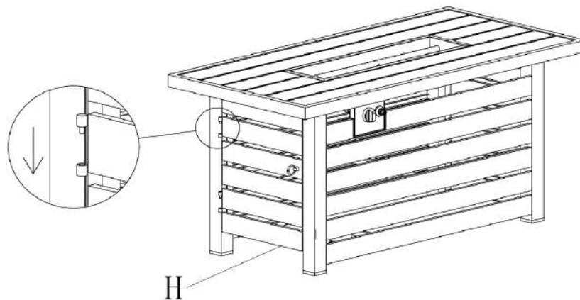
6. Turn over the Gas Fire Table, insert panel (H) to the door pivot.
