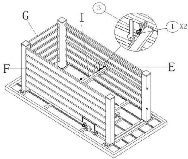
4. Attach stop lever (I) with panel (E) and panel with window (F) together using 2 pcs of Bolts(①) with Allen Key(③). Pls do not fully tighten.
