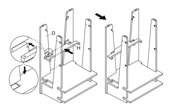
Step 6. Attach lower shelf (part C) to assembled unit (parts D, F & H).
