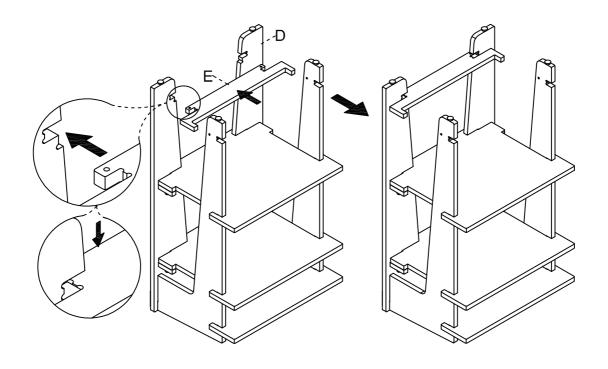
Step 8. Attach lower shelf (part C) to assembled unit (parts D, E & F).
