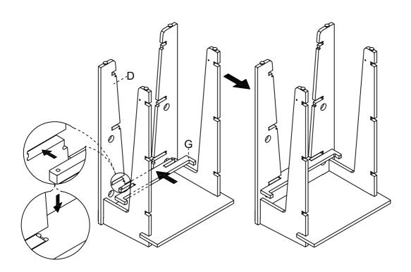
Step 4. Attach middle shelf (part B) to assembled unit (parts D, F & G).
