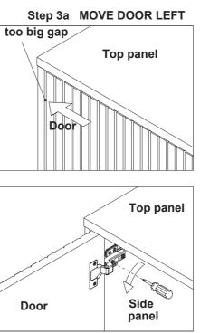
Turn the screw clockwise a little as shown to make the gap smaller
