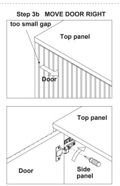
Turn the screw counterclockwise a little as shown to make the gap bigger
