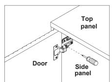
Loosen or tighten the screw indicated a little to adjust the gap between the door panels, adjust the hinge to the right position (see step 3a & 3b).
