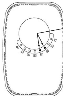
Pins are shown installed at 60 and 65°. The temperature setting range is limited between these two temperatures.
