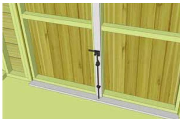
**77.** Once the Cane Bolt is attached, close doors and mark a hole in the stop to accommodate the bolt. You can bang the top of the bolt using a hammer and a block of wood to prevent damage. Once complete, open doors and drill hole where previously marked with 1/2" bit.
