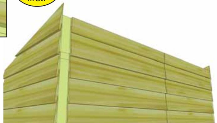
**28.** Position and secure 2nd Wall Extendor Panel as per **Steps 26 & 27**. Additionally, attach to first Extendor with 2 - 2 1/2" screws.
