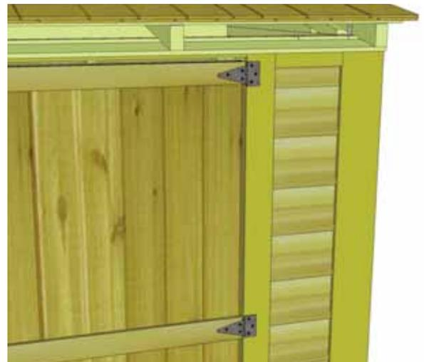
**63.** Now secure the Double Doors. Starting with **Right Side Door**, position so there is a 1/2" gap on bottom, and approximately 3/8" on the side. Use a spare piece of siding or shingle to shim door in place at the bottom. Using 2" black screws, secure bottom hinge to Door Trim. **Hint:** Do not attach all the 2" screws until both doors are positioned correctly. You can use a Screw Driver to tighten screws completely so you don't over tighten.
