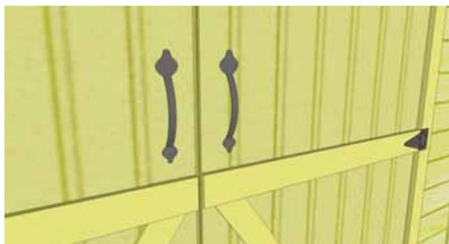
**78.** Attach **Door Handles**. Handles are positioned on top section of each door and mounted with 3/4" Black Screws.
