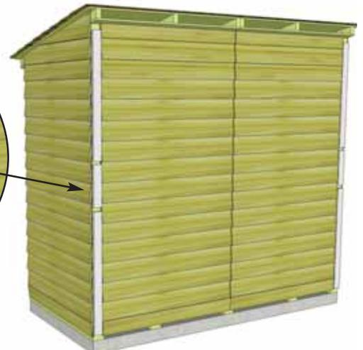
**53.** Position and attach Corner Filler Trims in the rear as per **Step 52**. There is an additional 10" long **Rear Center Corner Filler Trim** that you will need to center and attach as well using 2 - 1 1/2" nails.
