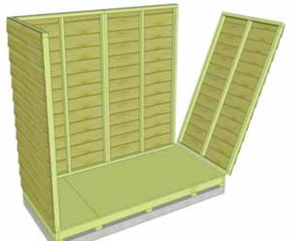
**14.** With Rear Wall Panel in place, position other side wall panel on floor as per **Step 10 & 11**.
