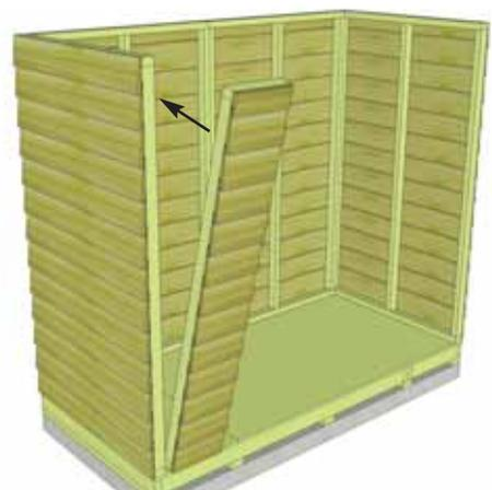
**15.** Secure side wall panel to rear wall panel as per **Step 12**. Next, locate a **Narrow Wall Panel** and position in front corner.
