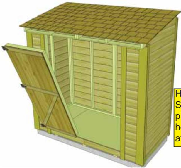
**Hint:** Use Shim Shingle or extra piece of siding to help space Doors at top and bottom.
