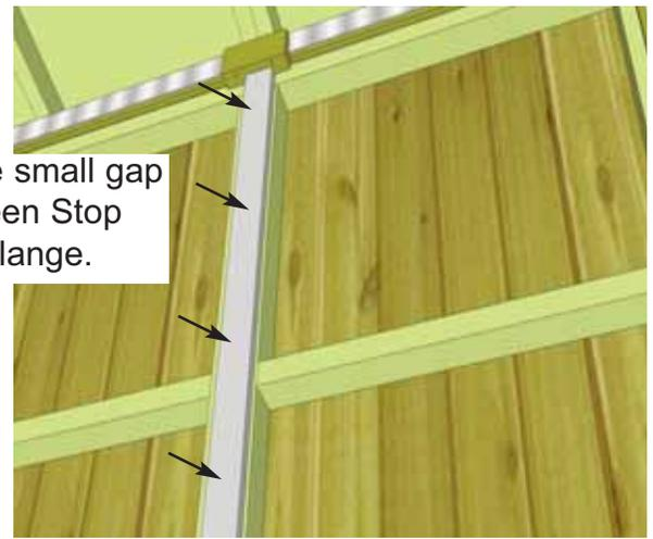
**75.** Position and attach **Interior Vertical Door Flange** (1/2" x 2 1/2" x 70") on inside door frame (**left door from outside/right from the inside**) using 6 - 1 1/4" screws. Position on inside edge of left door frame so Flange overlaps right door frame by about 3/4".
