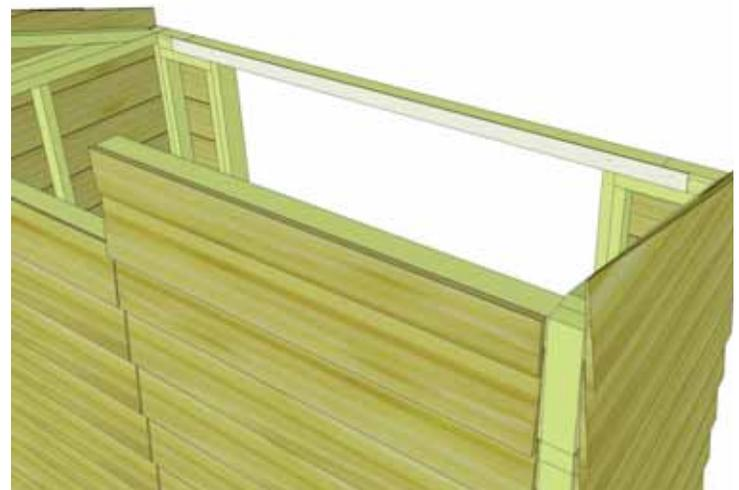
**27.** With 2x3 wall framing aligned, attach Wall Extendor to both the Angled Wall Extendor framing and the rear wall framing with 5 - 2 1/2" screws.
