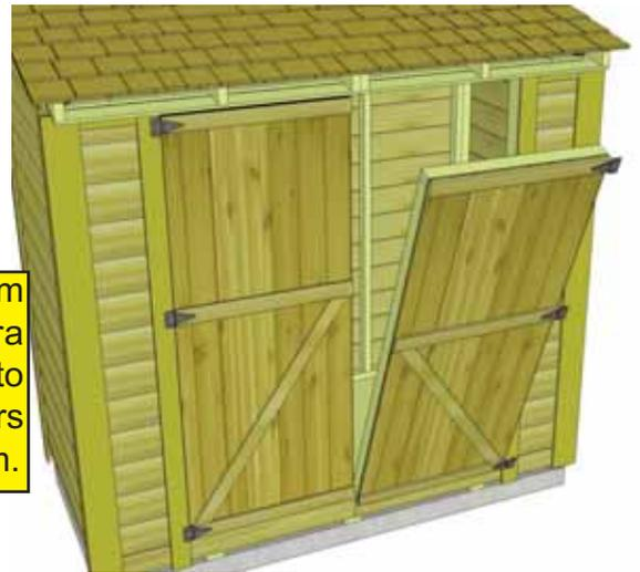
**62.** With Hinges attached, position doors in opening. You will need some assistance to hold doors in place.
