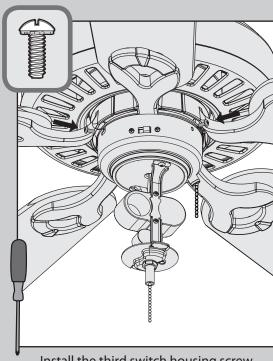
Install the third switch housing screw.
