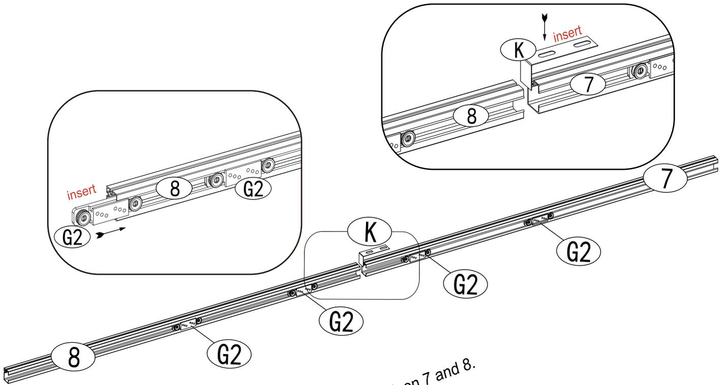
Corresponding to the position of the hole, stuck on 7 and 8.
