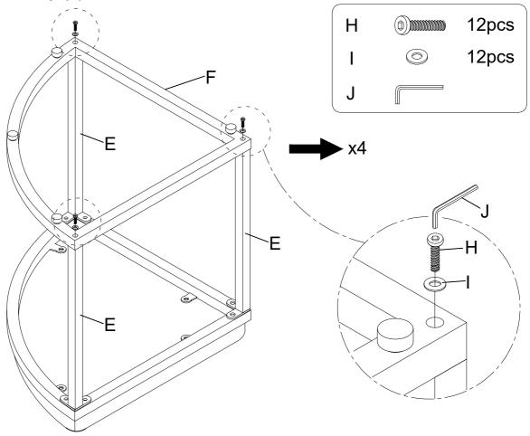
6 Adjust any parts out of alignment and tighten all bolts from step 4 through 5.
