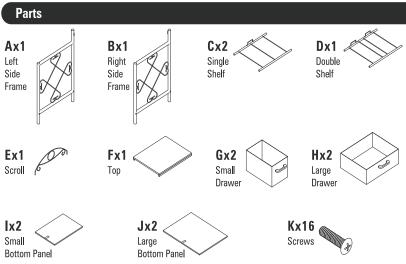
NOTE: Finger tighten screws until fully assembled, unless instructed to "tighten fully".
