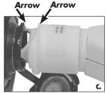
**8.** Push **EXPRESS PUMP**® firmly into valve (d). Do not force. Twist pump to lock into place (e). Turn on switch to begin inflating (f).
