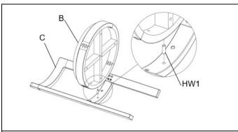
STEP 1: ATTACH BACK LEG FRAM (C) AND SEAT FRAM (B) BUY USING STEP 2: PUT THE WASHERS ON THE BOLT IN THE DOWEL (HW1)
