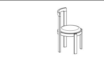
STEP 5: PUT THE CHAIR UPRIGHT AND MAKE SURE ALL LEGS ARE LEVEL, THEN FIRMLY TIGHTEN BOLTS WITH ALLEN KEY WHILE THE CHAIR IS UPRIGHT AS PICTURED ABOVE
