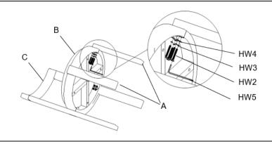
STEP 4: INSERT THE FRONT LEGS (A) AND SCREW IN THE BOLTS BUT **DON'T** TIGHTEN COMPLETELY
