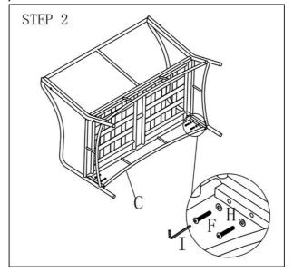
3. Locate the Chair Seat(C) to the Chair Back(D) by the pre-drilled threads. Fasten Bolts(F) with Washers(H) by using Allen Key(I) to combine chair seat and chair back together. 3 bolts should be fastened totally. (Step 3).
