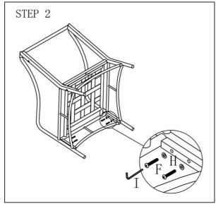
3. Locate the Chair Seat(C) to the Chair Back(D) by the pre-drilled threads. Fasten Bolts(F) with Washers(H) by using Allen Key(I) to combine chair seat and chair back together. 2 bolts should be fastened totally. (Step 3).
