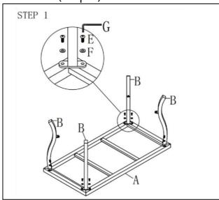
2. Locate Table Rack(C) to 4 Table Feet(B) by the pre-drilled threads. Fasten Bolts(E) with Washers(F) by using Allen Key(G) to combine table rack and table feet together. 4 bolts should be fastened totally, 1 for each corner of the rack. Now fasten all bolts tight. (Step 2)
