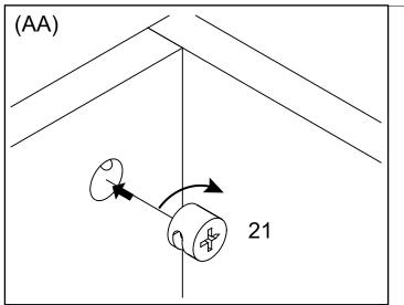
Pre-installation instructions There will be multiple No. 21 accessories in the follow-up. Do not repeat a single description in the installation step. Here, we will explain in a unified way. When installing No. 21 accessories, you need to align the top of No. 23 accessories at the back end of No. 21 and turn No. 21 clockwise, like an arrow. The marked direction. This description is numbered (AA) and then unified as (AA)
