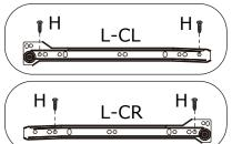
Fix rail(L) to two board 2 and 16 with screw(H) as shown.
