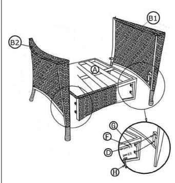
Position Arms L & R (B1 & B2) to their corresponding holes on the Seat frame (A) and use Plain washer (G) and Lock washer (F) and tighten long Allen Bolt (D) using Allen wrench (H)
