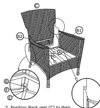
2. Position Back rest (C) to their corresponding holes on Arms L & R (B1 & B2) then use Plain washer (G) and I ock w(F) and tighten sho Allen Bolt (E) on bottom rail using Allen wrench provided (H)
