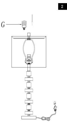
Step2 Insert the bulb(G) into the socket(C).
